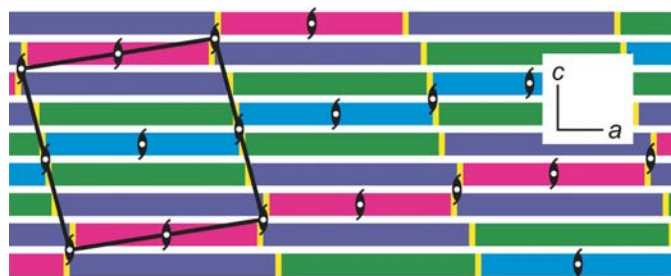
Figure 14 Stacking of the layer of modulated As nets of \text{GdAuAs}_2 along [001], color code according to Fig. 12. The positions of the twofold screw axes are highlighted, the monoclinic repetition unit with a' = 62.84 , b' = 4.060 , c' = 64.12 Å, \beta' = 95.49^\circ is emphasized with bold black lines.
